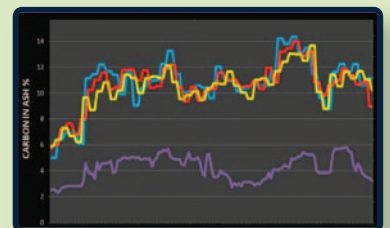
3-Probe Carbon Cross Duct Trend gives Confidence in Combustion Performance
